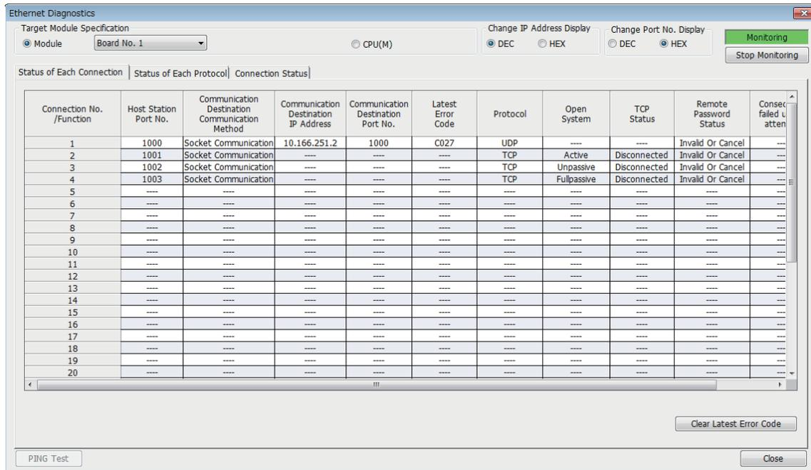
The following functions can be used in the "Ethernet Diagnostics" window for the FX5-ENET.
