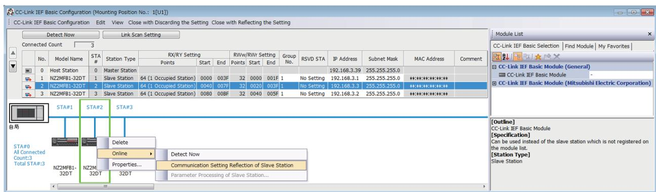
Follow the operating procedure below to use the automatic detection of connected device.
